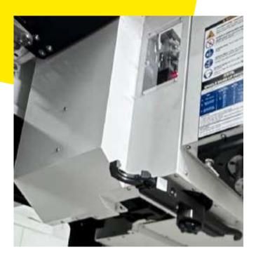
Automatic Tool Changer 16 positions BT30 | Power Drawbar Arm type
